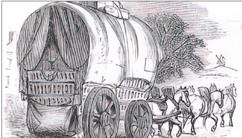
A long wagon. Note the wide wheels to help the wagon ride the muddy and broken road surface.
